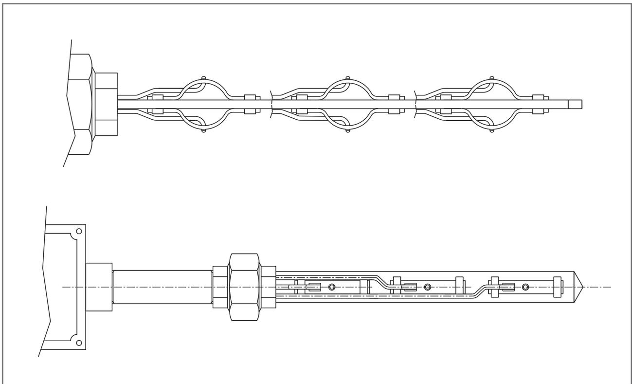
Spring loaded (with the help of 'S' spring or leaf spring) thermocouples located at various points mounted on a plate enclosed in a protecting tube as shown above. The springs ensure proper contact with the protecting tube. As many as 33 points assembly was supplied as import substitution for a reputed fertiliser plant.
