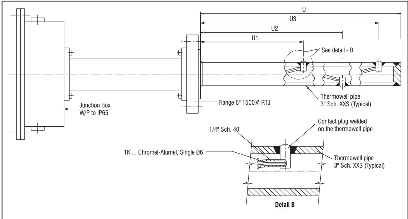
Thermocouples at various levels inserted in individual guiding tubes which in turn are welded to outer protecting tube as shown.
