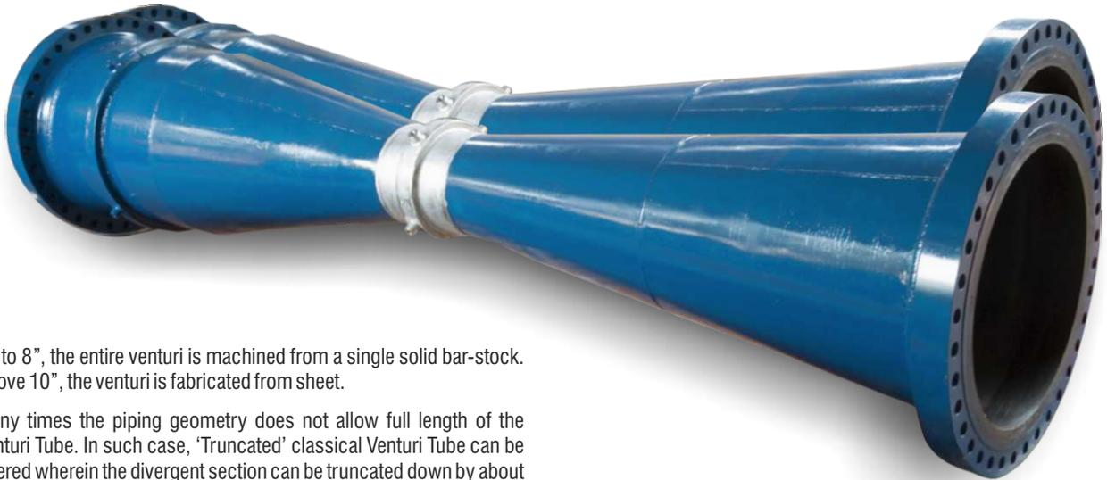
Up to 8", the entire venturi is machined from a single solid bar-stock. Above 10", the venturi is fabricated from sheet.
