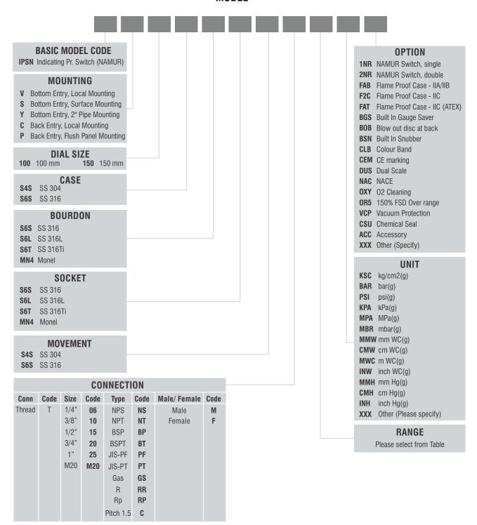
e.g. For 1/2"NPT(M), Code: **T15NTM** For M20x1.5 (F), Code: **TM20CF**
